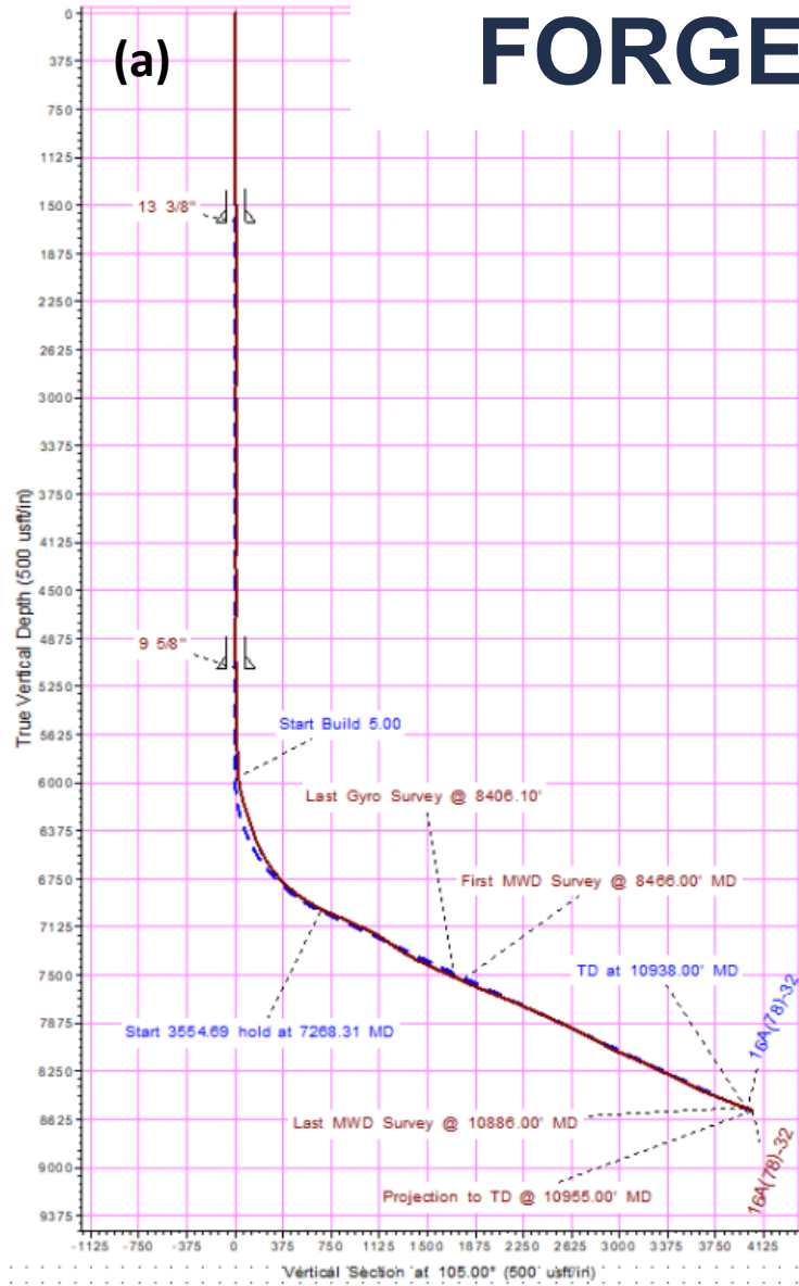
Figure 2. (a) Directional profile (approximate elevation view) 1 ; (b) Plotted deviation survey in Spotfire
